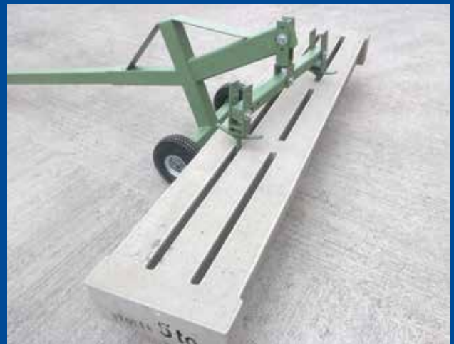
Laying dolly for cattle slatted floors
