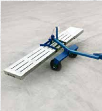
Laying dolly for pig slatted floors
